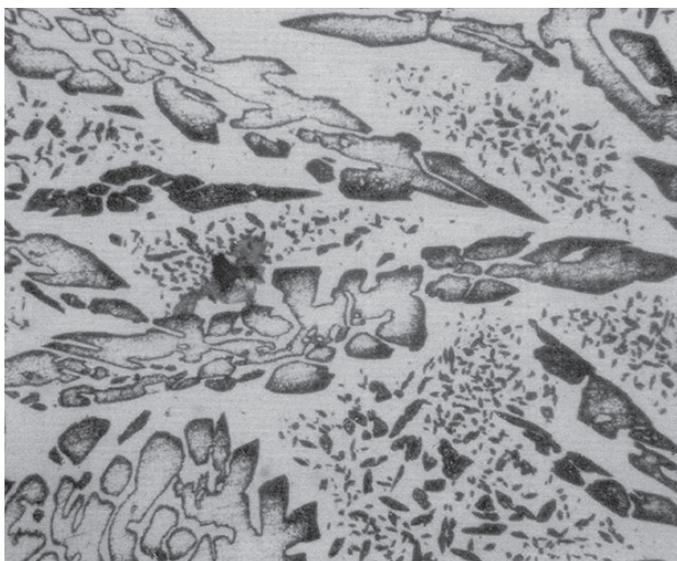
This photo is an optical microscopic view of WCD4™ at x250 magnification. The microstructure consists of primary and secondary austenite grains embedded into the ferritic matrix.
